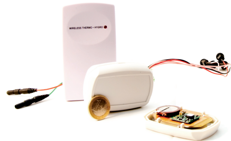
Fig. 13. Packaged 2.45GHz remote RF battery charger and COTS 433MHz wireless temperature and humidity sensor. 433MHz base station not shown.
