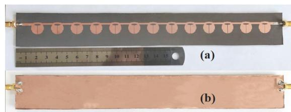
Fig. 13. Photograph of the manufactured microstrip CP LWA. (a) Top layer. (b) Bottom layer.
