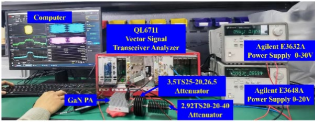
Fig. 6. (a) Synoptic diagram with respect to 3GPP EMC compliance standard and (b) photo of 5G communication EMI test platform.
